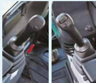
Proportional hand control lever for N&B piping (option) Precise proportional controls are integrated into the joystick for ease of operation.
